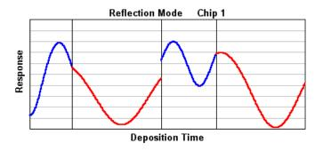
Note how the cutoff ratio for layer 2 utilizes the maximum value achieved by layer 1. There are two turning points for layer 3 but only one for layer 4. (If **Neglect initial turning point** is unchecked, layer 4 shows two turning points.
