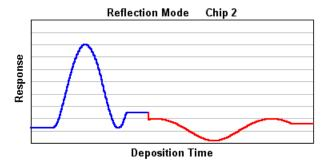
While design layer 4 (C2/L2) has good selectivity, a higher gain setting will be beneficial. Click **Edit...Options <Ctrl+O>** to bring up Worksheet Calculation Options (no need to leave the strip-chart dialog!) and uncheck **Same gain/offset** *for all layers* to enable variable gain settings (different values for different layers on a chip) and note that *Use current worksheet values* option is now enabled. Finally, change *Auto Level Type* to Initial.
