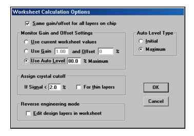
The worksheet re-appears with odd and even chips delineated with cyan and yellow background. The worksheet is now active (connected to its underlying data) and wavelengths can be edited. The Worksheet Options box can be activated without recalculation via **Evaluate...Calculation Options <Ctrl+O>**.
