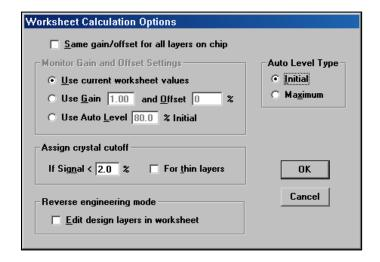
Return to the chart with **<F8>** and select **Setup...Single Layer <Ctrl+L>**. Press **<PgUp>** or **<PgDn>** to arrive at C2/L2. **Edit...Gain <Ctrl+G>** brings up the Monitor Gain dialog. Enter *Initial Level=60*, click **Set** to calculate gain/offset, and click **OK** to replot the curve.
