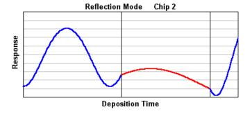
A far more dramatic change occurs in chip 2. The cutoff for layer 2 now utilizes its own maximum as well as the previous minimum from layer 1. The cutoff for layer 3 uses its minimum as well as the previous maximum from layer 2.
