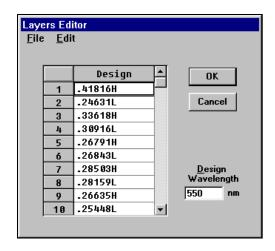
Layers are deleted with **<Del>** or by clicking **Edit...Delete Row <Ctrl+D>**. Rows are inserted with **Edit...Insert Row <Ctrl+I>**. A design text editor resembling DESIGN's groups mode editor is accessed via **Edit...Text <Ctrl+T>**.
